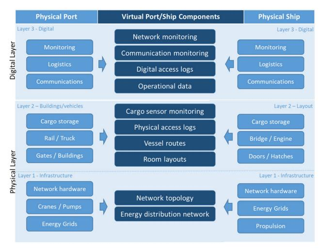
Figure 3 Maritime virtual and physical components for ships and ports categorized into layers.
