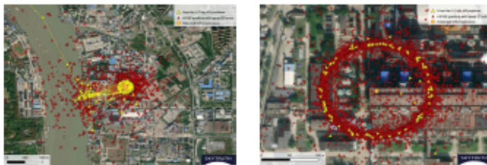
GPS interference can be pinpointed based on the ring of false AIS positions (200 meters in diameter). Positions in the ring reported speeds up to 11 knots and a course going counter-clockwise around the circle.
